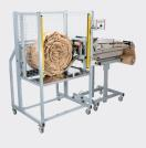
The Coiler is a bolt-on solution designed to be used in conjunction with the Packmaster™ Pro system in order to automate the process of producing consistent, large quantities of highly protective paper coil.
