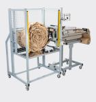
The Coiler is a bolt-on solution designed to be used in conjunction with the Packmaster™ Pro Fanfold system in order to automate the process of producing consistent, large quantities of highly protective paper coil.
